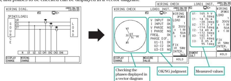
Checking the phases displayed in a vector diagram, OK/NG judgment, Measured values
